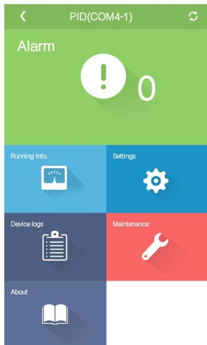
**Step 6** Tap **Settings** to access the settings screen and set PID module running parameters, as shown in [Figure 4-8](#).
