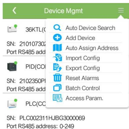
**Step 4** Tap **Monitoring** on the SmartLogger home screen to access the device monitoring screen, as shown in [Figure 4-6](#).
